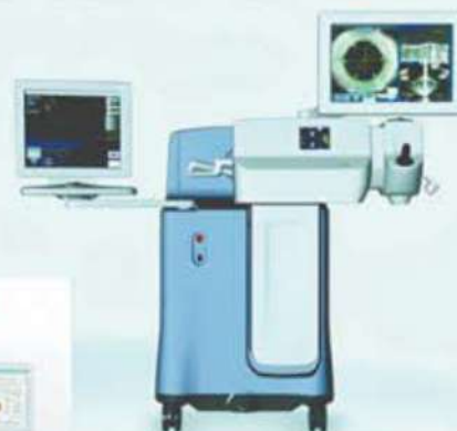
FLACS (Femto Laser Assisted (Bladeless) Cataract Surgery) by The LENSX laser system
